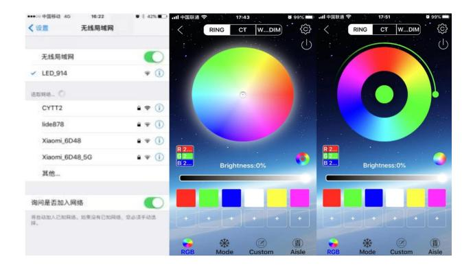
Once the connection is successful, exit the mobile phone's settings, open the "LED Wifi" app, and the color ring control interface will appear, allowing you to perform the corresponding mode operations.
