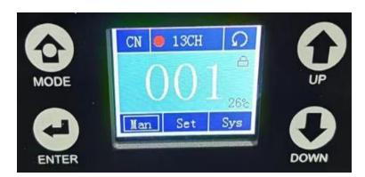
Press MODE to unlocked interface and input 111 to unlock
